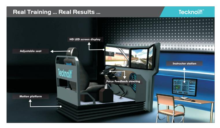
**TecknoSIM Light Vehicle Simulator** is an **advanced training tool** that provides real life training experience to both **novice and experienced drivers**. The simulators immerses the drivers in **real life driving scenarios** under complete safety. TecknoSIM Simulators are beneficial for driving institutes, research institutes, vocational training institutes and logistic companies. The simulator assists in improving **productivity, safety and cost efficiency.**
